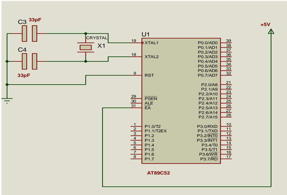
Figure 5: Essential Circuitry to the AT89C52 Micro-controller
