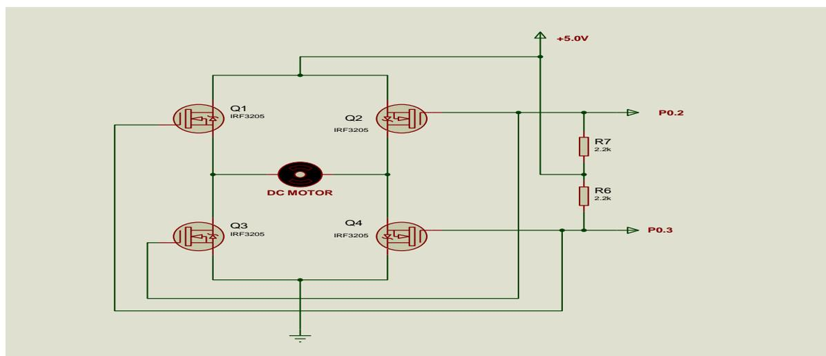
Figure 3: H-bridge circuit for driving DC motor.
