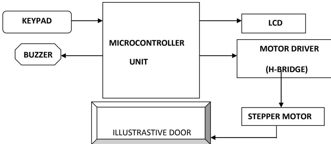
Figure 1: Block diagram of the security system.
