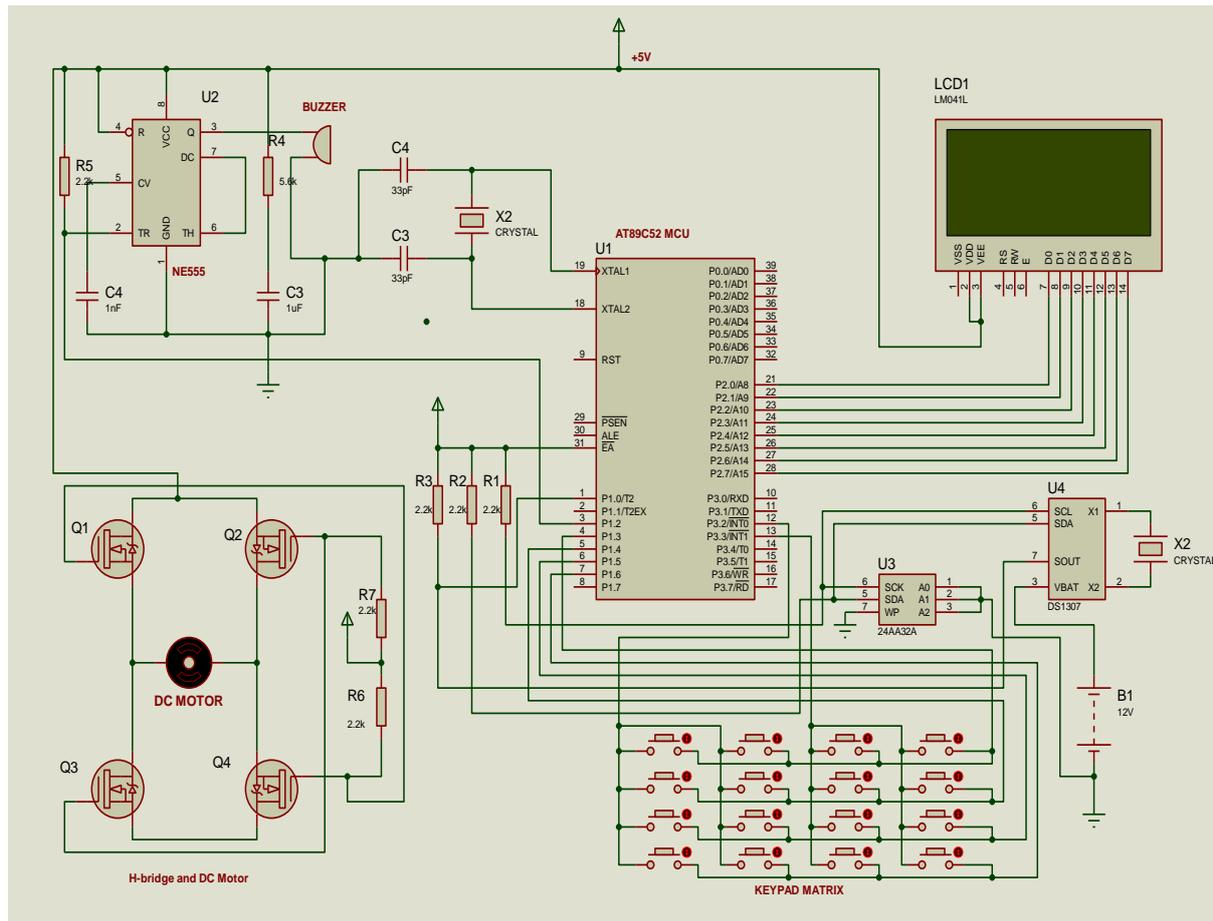
Figure 7: Circuit diagram for a password based door lock security system.
