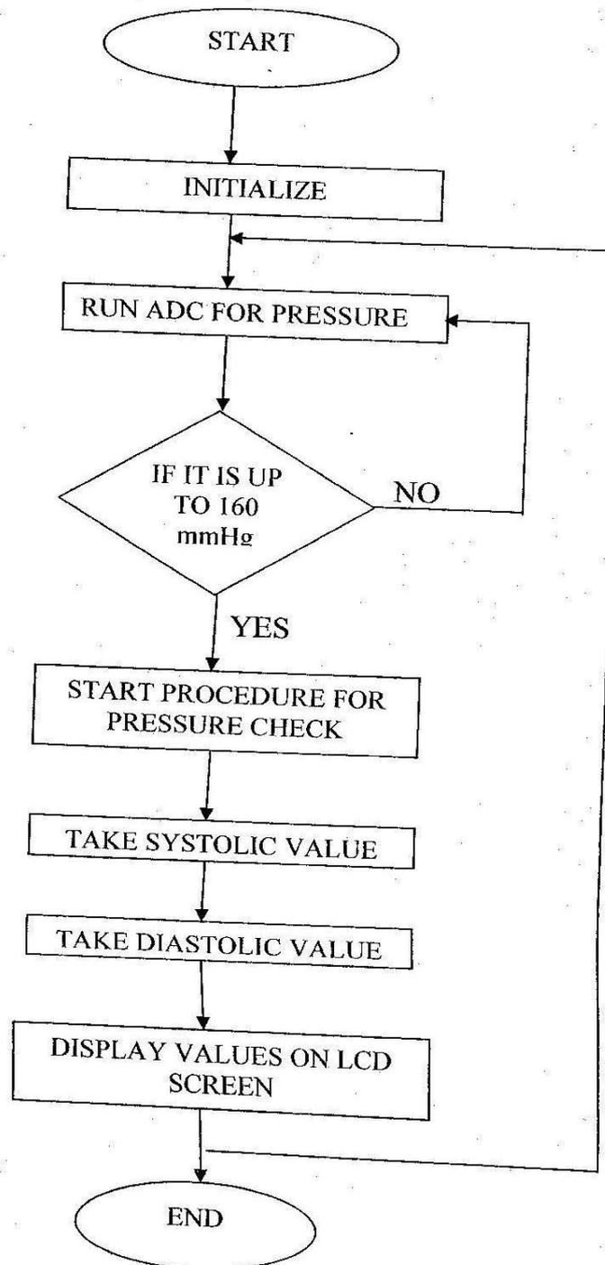
**Figure 2: Flow chart for a digital blood pressure monitor**
